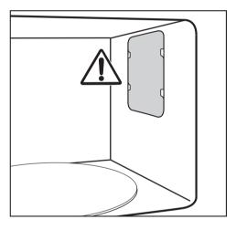
Do not remove the cover to the microwave outlet inside the oven, nor the film covering the inside of the door.
